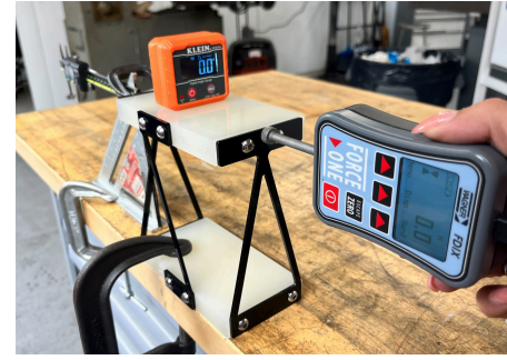
Our verification setup, consisting of the force gauge, angle gauge, and calipers.
